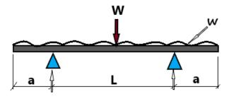
6. To determine the economical cross-section of a simply supported beam subjected to combined loading from the given two options - square cross section and circular cross section. Given, allowable bending stress, length of beam, magnitude of point load and intensity of u.d.l.
